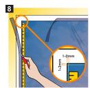
Using a Straight Edge, trim excess film leavin g a 1-2mm gap for any water residue to escape.
